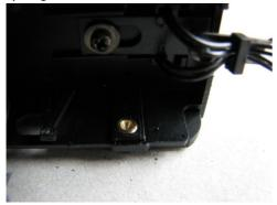
Shouldered pinpoint bearing inserted into axle hole.
