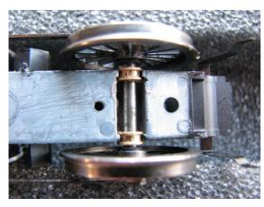
Keeper plate removed exposing axles and bearings.
