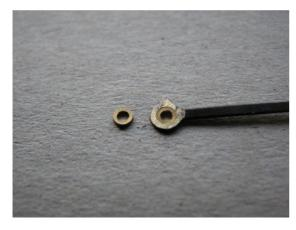
Bush inserted into rod ready for soldering.
